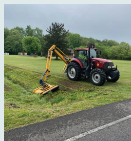
Boom mowing the drainage ditch along CR 538 Elk Road in Elk Township.
